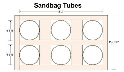
how you will slide the tubes into each hole. You will need to put the 1-5/8 screws through the tube and into the sides where it touches the boards on all four sides. There should be two screws at each spot. First, take your drill and pre-drill the 8 holes on each tube; one at 1" from the top and one at 2.5" from the top every 90 degrees. Now put the tube in the frame and put screws in each hole. The easiest way is with a right angle drill.
