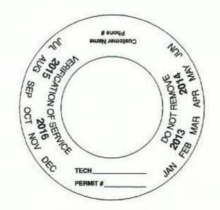
c. The collar shall include the following information. Month and year the service was performed, indicated by a perforation such as is done by a hand punch and name of the agency performing the maintenance or recharge.
