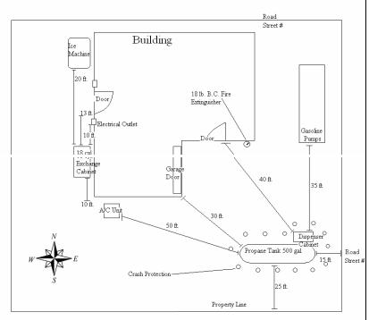
Installation of tank and piping as per NFPA 58 (2014), NFPA 54 (2012), and the International Fire Code (2015 Edition) Chapter 61
