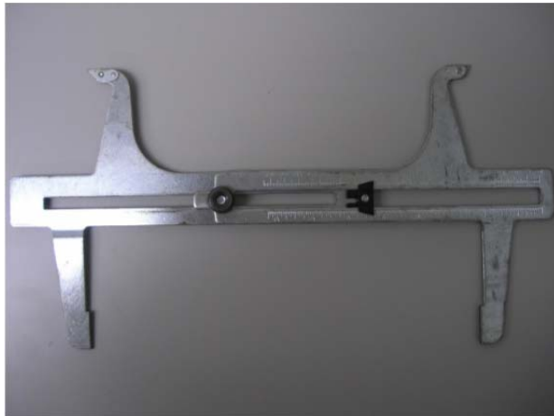
Brake Drum Gauge
