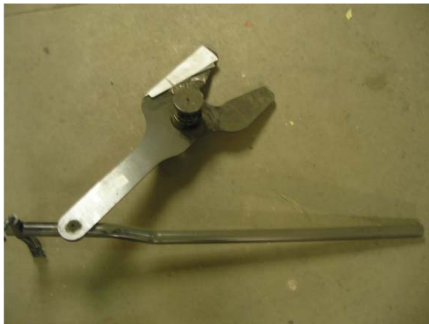
Fifth Wheel Jaw Tester (Heavy Duty Only)
