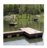
Floating Docks and Wheeled Piers attached to the shoreline must be located as near as possible to the center of the adjacent upland parcel and extend into the water at approximately a 90 degree angle to the shoreline.
